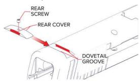
**NOTE:** Make sure that the installation procedure is made long before the threadlocker cures. After installation, allow a minimum of 8 hours for the thorough curing of the threadlocker.
