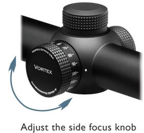
**Parallax** is a phenomenon that results when the target image does not quite fall on the same optical plane as the reticle within the scope. When the shooter's eye is not precisely centered in the eyepiece, there can be apparent movement of the target in relation to the reticle, which can cause a small shift in the point of aim. Parallax error is most problematic for precision shooters using high magnification.
