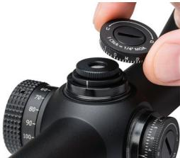
2. Lift dial off of scope. Orient dial to reposition the zero mark on the index line.
